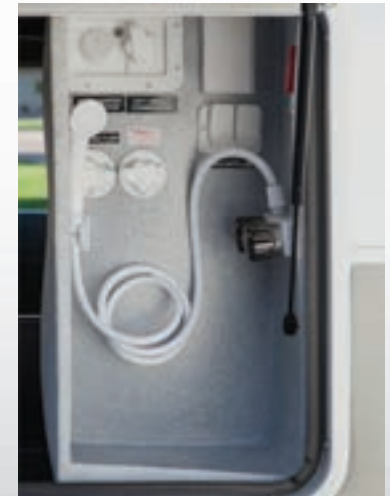
Exterior convenience center houses 110V outlet, cable and satellite hook-ups, hot and cold exterior shower and black tank flush
