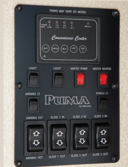
Convenience Center panel controls slides, awning, interior and porch lights, water pump/heater; shows battery/tank capacities
