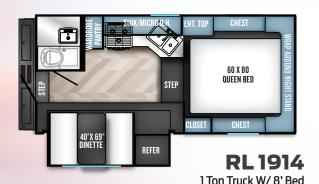
Ext. Length (with Ladder): 19'3" Ext. Width: 8'2" Floor Length: 10' Wheel Well Width: 48" Ext. Height (w/ Ladder): 9'9" Int. Height: 6'8" Dry Weight (Lbs.): 3493 LP Gas (Lbs.): 30
