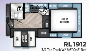
Ext. Length (with Ladder): 18'4" Ext. Width: 8'2" Floor Length: 9' Wheel Well Width: 48" Ext. Height (w/ Ladder): 9'9" Int. Height: 6'8" Dry Weight (Lbs.): 3261 LP Gas (Lbs.): 30 Fresh Water (Gal.): 45 Gray Water (Gal.): 20 Black Water (Gal.): 20
