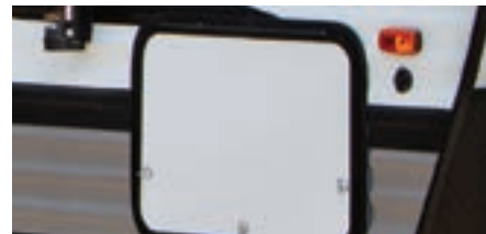
Radius compartment doors are silicone sealed to protect from the elements.
