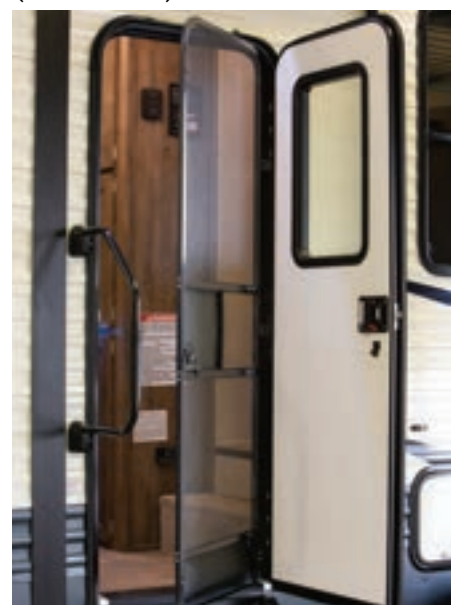
Friction hinge door with window and kick plate
