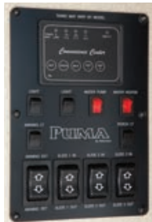
Convenience Center shows battery/tank capacities. Controls slides, awning, interior/porch lights, water pump/heater
