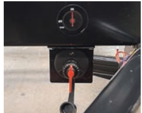
Seafo battery isolator switch prevents power drain. Operates by removable key.
