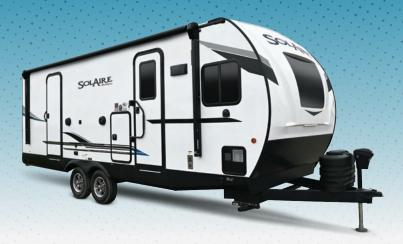
The Ultra Lites are the result of superior design and modernization. Striving to meet all the customer's demand this trailer provides a smooth ride with independent suspension axles, aluminum superstructure frame for light weight towing and barreled ceilings for a more spacious interior.
